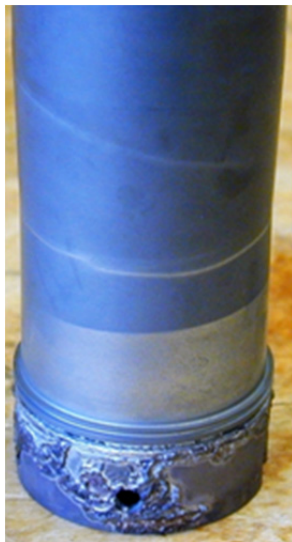
Figure 5.—SN18 heater head: Vacuum furnace de-brazing attempts failed to separate the heater head from its permeometer mounting flange.
